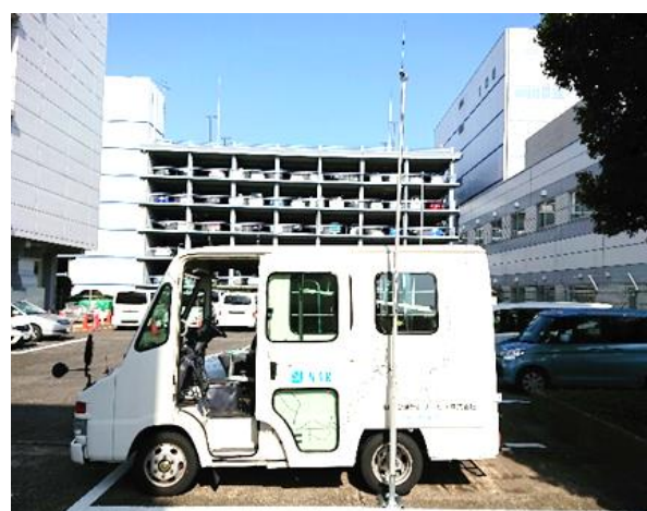
Figure 9 Mobile base station of TETRA system
