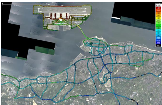
Figure 7 Radio wave signal strength and around Chubu Centrair International Airport
